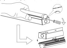
3). Fix the rear aluminium casing to the wall/ceiling.
