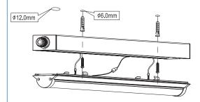
5). Assemble the lamp body on the Aluminum casing.
